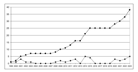
Figure 1. History of the ISS collision avoidance actions.
